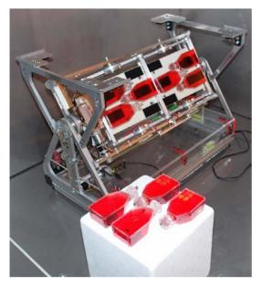
**Figure 8.** Random positioning machine (RPM). The RPM consists of a gimbal-mounted platform, which rotates samples continuously around two perpendicular axes. Samples were closed with a custom-made silicone plug and a stainless steel pin and subsequently fixed with Velcro onto the RPM. The Lucerne School of Engineering and Architecture developed the RPM.
